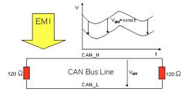
The CAN bus termination must be set by software on Object 2102h.
