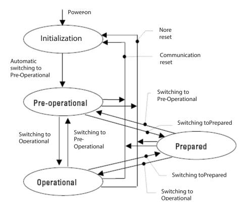
**Initialization:** This is the initial state after the power supply is applied, following a device Reset or Power ON. The node automatically enters the Pre-operational state once it has run through the Reset and Initialization routines. The LEDs display the momentary status.
