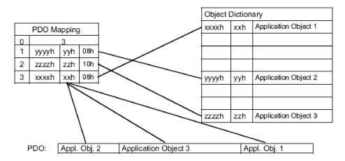
Application Object 2 occupies Byte 1 (08h) in the Transmit PDO. Thereafter follows Application Object 3 with a length of 16 bit (10h = 2 bytes) and finally Application Object 1 with a length of 1 byte. In total, 32 bits are occupied in this PDO.
