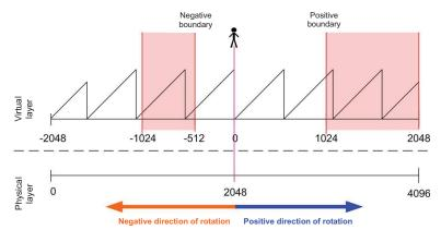
If, during the operation of the system, one of these critical areas is reached, a correction must take place, which will shift the current position on the virtual layer so that the physical position is located again outside of the critical area. This will create a virtual position on the user layer, and the encoder will always be in the safe area.
